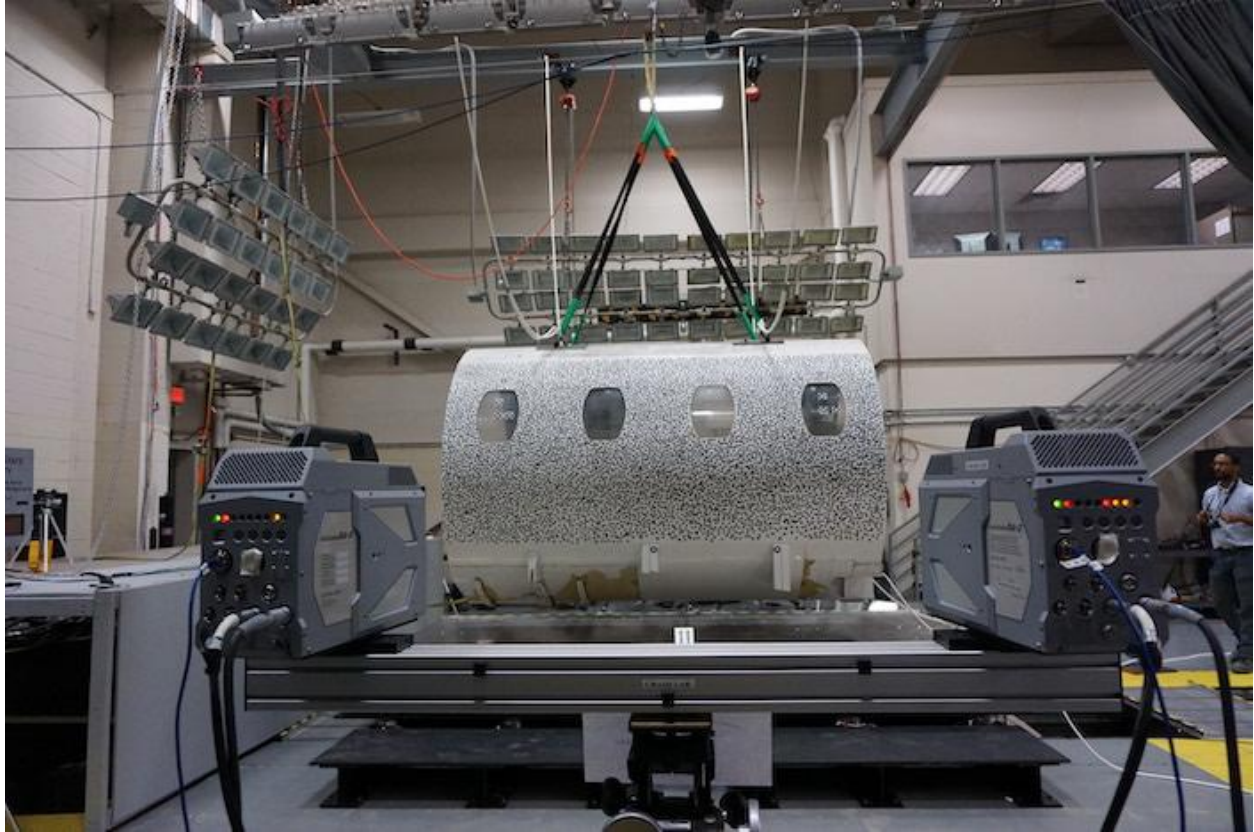
Figure 35: DIC testing on an aircraft fuselage (Roper)
