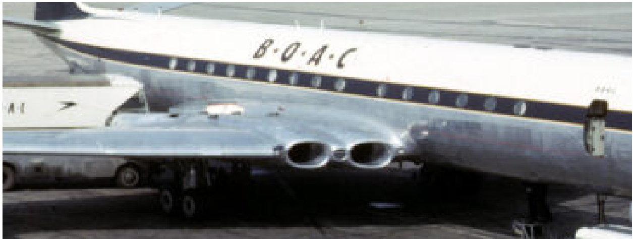
Figure 2: Havilland DH 106 Comet airplane after windows were modified to be circular (Beresnevicius and Mickeviciute)
